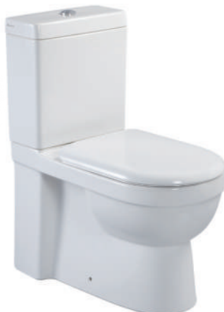
LAGINA Item Code : 140500100405 Washdown One Piece Closet Size : 675 x 370 x 800 mm P-trap, 180mm Roughing-in
